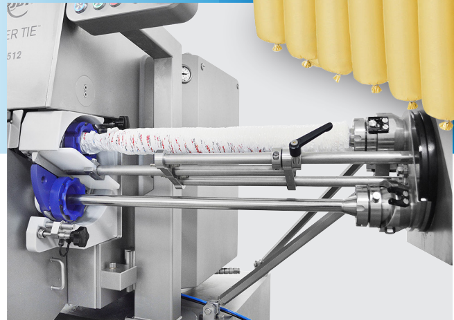
Fast casing changes thanks to parallel turret
