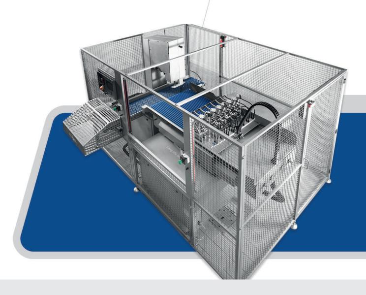
The RB-1 Automatic Bandsaw single & double cut has been designed to work automatically and precisely, cutting accurately the predetermined measures of any frozen or fresh product, either meat, fish, or vegetables.
